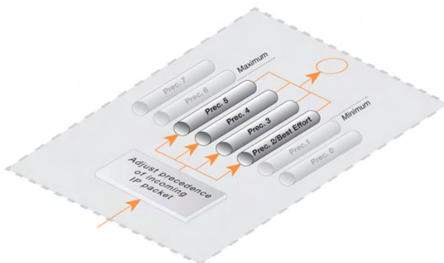
Figure 10.3. Minimum and Maximum Pipe Precedence.
